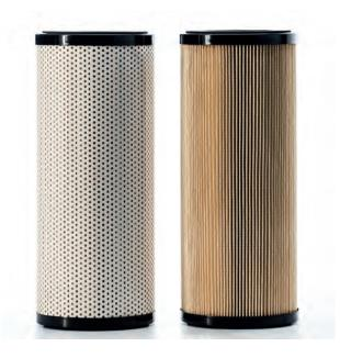
The Facet M Series high efficiency pleated paper filter cartridges are excellent for removing solid contaminants such as rust, dirt, scale, granular and other types of solids from fuels. Media with high efficiencies throughout the life of the cartridges are available to the aviation market in ratings of 0.5 to 15 nominal microns. These cartridges can be provided with either a perforated paper or expandable metal outer wrap if required.
